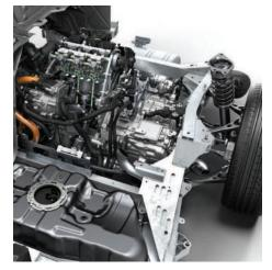
continuous electric power to the wheels in two different ratios to meet the performance targets.
