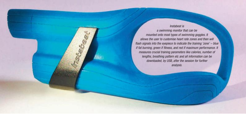
selecting the correct materials that would bond well to each other and thus create water tight seals. Effectively the product is electronics moulded into low hardness plastic. In addition to being water tight the product had to be flexible to adjust to any swimming goggles, but rigid enough to hold firm against the swimmers head for good heart rate measurement. So the hardness range of the plastic further limited the material options."
